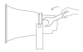
2 Fix mounting bracket on the flat surface.
