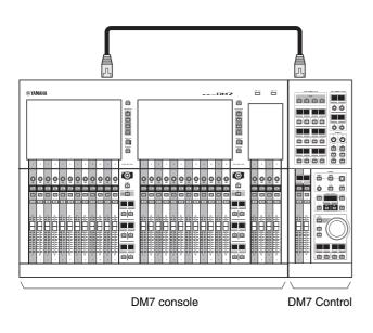
You can link up and affix this product to the DM7 console using joint metal brackets. ("Linking with the DM7 Console"  $\rightarrow$  page 12)
