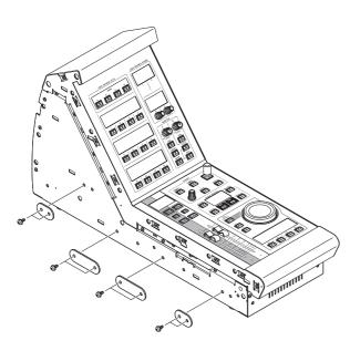
**2.** Remove the side pad of the DM7 console from the side panel to which you plan to attach this product.
