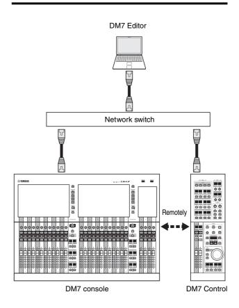
You can use this product (which is connected via a network cable) in another location on the network, remote from the DM7 console.
