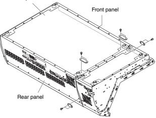
**5.** Turn the linked DM7 console and this product back to the original position, and then attach the side pad to this product.
