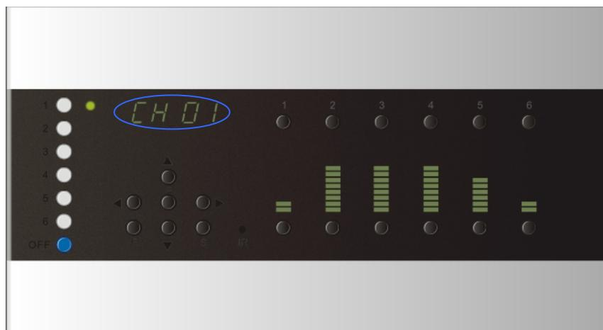
2. Press **【S】** shift to channel 7 ~ 12, the screen will display as below. **【CH1- CH6 UP/ DOWN】** can adjust the dimming value channel 7 ~ 12 correspondingly.
