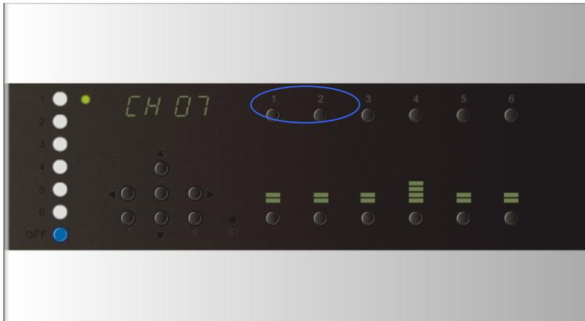
While edit the dimming value of channel 4, the screen will display as
