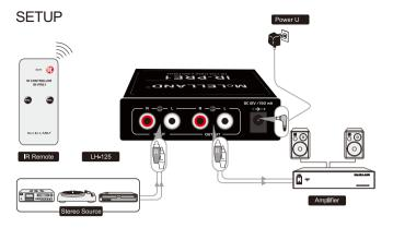
Please turn the power off all the units when the first time to make connections or change any existing connections.
