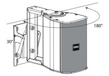
The brackets allow a rotation on the horizontal plane of  $180^{\circ}$  to step of  $15^{\circ}$  and a tilt on the vertical plane of  $30^{\circ}$  to  $8^{\circ}$  step.
