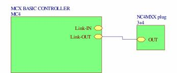
During operation, the NC4MXX plug must be connected to the last controller in chain
