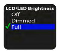
Press **<DOWN>** or **<UP>** to choose the brightness of LCD display and LED state
