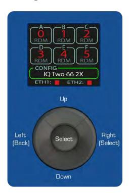
ProPlex IQ Two can be configured locally on the unit by using the keypad or remotely through the Ethernet port by accessing the built-in web page with a web browser or with the ProPlex Software.
