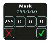
Press **<UP>** or **<DOWN>** to change value for each highlighted window. Press **<LEFT>** or **<RIGHT>** to navigate selection window. Press **<DOWN>** and then **<LEFT>** or **<RIGHT>** to decline or confirm, **<SELECT>** to accept changes.
