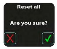
By pressing any of three default settings, another window will pop up to confirm or decline changes. Navigate to decline by pressing **<LEFT>** and confirm by pressing **<RIGHT>**.
