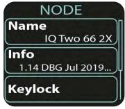
Press **<SELECT>** or **<RIGHT>** to enter the Node Setup submenu or **<LEFT>** to return to the home screen.
