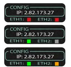
At the bottom of the home screen are located two indicators. **ETH1** and **ETH2** indicates status of the two Ethernet ports located at the back of the unit.
