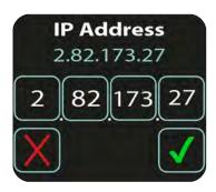
Press **<UP>** or **<DOWN>** to change value for each highlighted window. Press **<LEFT>** or **<RIGHT>** to navigate selection window. Press **<DOWN>** and then **<LEFT>** or **<RIGHT>** to decline or confirm, **<SELECT>** to accept changes for the IP address.
