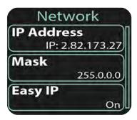
Press **<SELECT>** or **<RIGHT>** to enter the Network Setup submenu or **<LEFT>** to return to the home screen.
