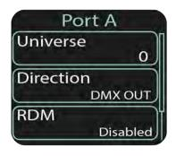
Press **<SELECT>** or **<RIGHT>** to enter the Port submenu or **<LEFT>** to return to the home screen. Select any of six ports to set the desired values.
