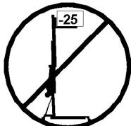
3.15 - The minimum load to avoid problems regarding the breaking mechanism is 25Kg. Without this load the brake will not work.
