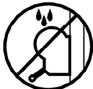
3.14 - Do not grease or lubricate the winch's breaking mechanism. The brake disks have been greased with a special heat and pressure resistant solution. Other products should not be used to avoid negative effects regarding the braking mechanism.
