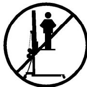
**3.1** - The HDT-08 is a machine designed to elevate loads upwards in a vertical direction. It should NEVER be used as a platform to elevate people.
