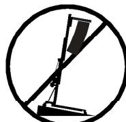
**3.2** - Only place the lift on hard, flat surfaces always checking that it is in a vertical position by using the bubble level indicator found on the base section. Adjust the outrigger stabilisers (Q) by turning the cranks to level if necessary. NEVER use wedges or other foreign objects to balance the lift.
