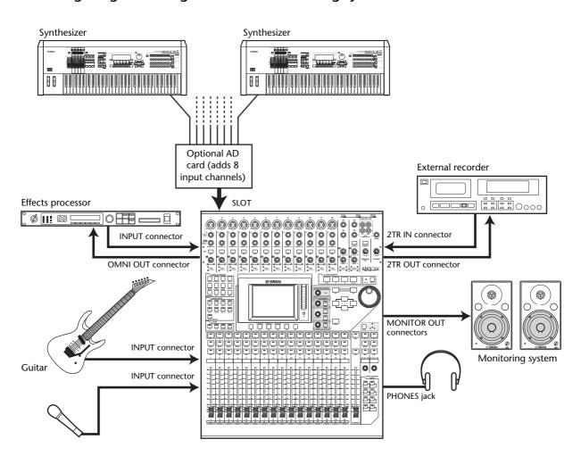
This illustration shows a simple system with 16 analog channels using the 01V96i's INPUT connectors 1–16. If an optional AD card (such as the MY8-AD or MY8-AD96) is installed in the slot, up to 24 analog channels can be mixed.
