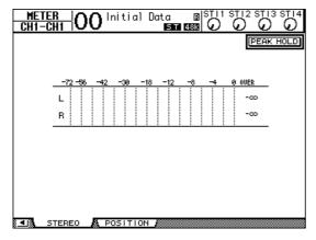
If you selected the CH1-32 page or the Master page, use the MASTER MODE parameter to select one of the following three metering signal types:
