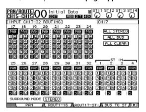
**8.** For each Input Channel 17–24, make sure that the S button is on and the 1–8 buttons are off, and use the PAN section to adjust the panning of the monitor signals as necessary.
