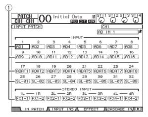
Inputs and Slot channels that are currently assigned to Input Channels are shown in the parameter boxes (1) beneath the channel numbers. The parameter indicators are explained below:
