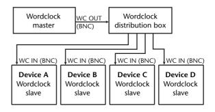
If the external devices do not have wordclock in and out connectors, you can use the clock information included in the digital audio signals. In this case, digital audio signals and wordclock signals are transferred via the 2TR OUT DIGITAL and 2TR IN DIGITAL jacks or via the digital I/O card installed in the rear panel slot.
