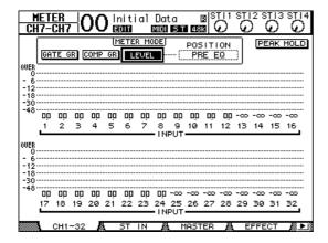
11. Play back the DAW, and adjust faders 1–8, [MONITOR OUT], and [PHONES] to set an appropriate level for the monitor signals.
