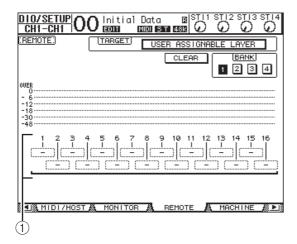
**4.** Select the channels you wish to assign to the User Assignable layer using the 1–16 parameter boxes (1).
