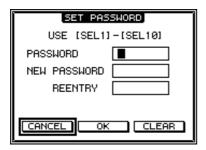
Enter the current password in the PASSWORD field, and a new password in the NEW PASSWORD field. The factory default password is "1234." Enter the new password again in the REENTRY field located below the NEW PASSWORD field. Move the cursor to the OK button, then press [ENTER] to change the password.
