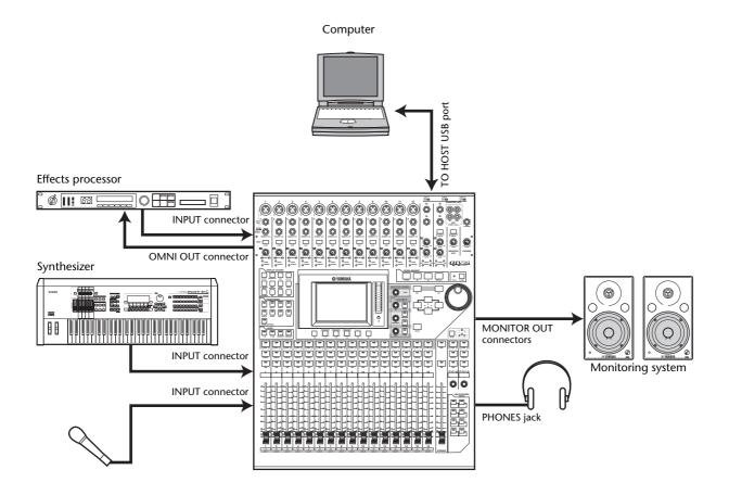
In this system, the 01V96i is connected to a computer-based DAW (Digital Audio Workstation). This allows the 01V96i to be used as an audio interface with 16-channel input and output. The 01V96i's remote functionality can also be used to perform locate and transport operations on the DAW, and to edit its parameters.
