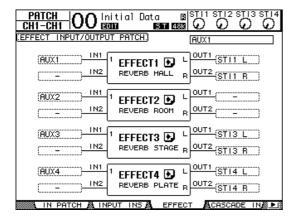
This page enables you to patch the inputs and outputs of Effects processors 1–4. By default, Aux Send 1 is patched to the input of Effects processor 1, and the output of Effects processor 1 is patched to ST IN Channel 1 L and R, as shown in the diagram above.
