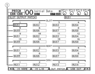
Signals that are currently assigned to the output connectors are shown in the parameter boxes (1) underneath the connector numbers. The parameter indicators are explained below:
