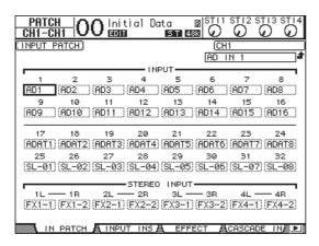
By default, signals from the instruments or mics connected to INPUT connectors 1–16 are sent to Input Channels 1–16. Input signals from the ADAT IN connector are sent to Input Channels 17–24, and input signals from the slot are sent to Input Channels 25–32.
