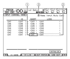
Channel IDs, Short names, and Long names are listed from left to right on the page. You can specify Short names in the parameter boxes (1) in the center column, and Long names in the parameter boxes (2) in the right column.
