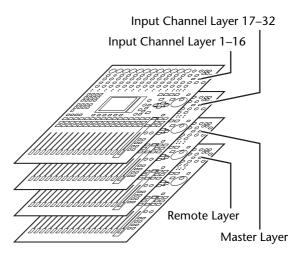
The currently-selected layer determines the function of the channel strip, [SEL] buttons, [SOLO] buttons, [ON]
