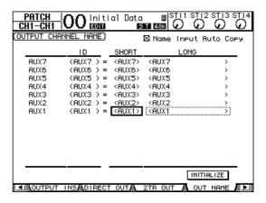
The procedure for editing the names and using the Name Input Auto Copy check box and the INITIALIZE button is the same as on the In Name page.
