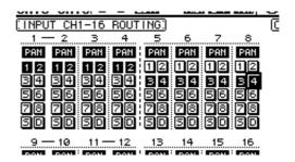
**4.** Press the [PAN/ROUTING] button repeatedly to display the Pan/Route | Pan page.
