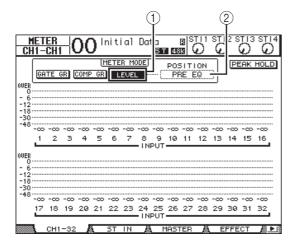
**4.** Make sure that the LEVEL button (1) is turned on in the METER MODE section.
