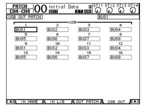
The parameter boxes underneath each number indicate the currently-assigned signal routing. The meaning of these indicators are explained below.
