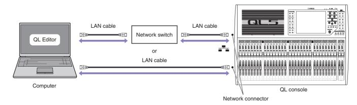
**NOTE** You cannot simultaneously control one QL unit from two computers running QL Editor. However, you can control the QL unit using QL Editor on a computer along with the QL StageMix application installed on an iPad that is connected via WiFi.
