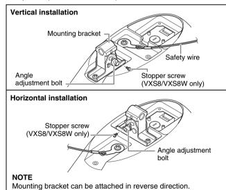
2 Set the desired vertical angle of the speaker. Loosen the angle adjustment bolt with the supplied hexagon wrench, adjust the angle of the speaker, and tighten the angle adjustment bolt to fix the speaker (indication of torque: 8 N·m).
