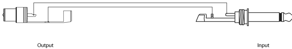
Cable to unbalanced input from RCA output. RCA and TS connectors.
