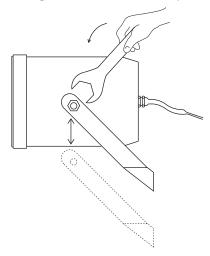
2 Fix mounting bracket on the flat surface.
