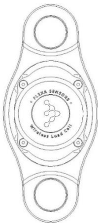
Fig. 15 – DynaCell lastcelle – batteriside – stålskruer
