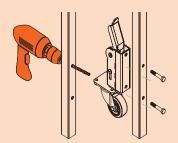
Drill holes into your stage deck to mount the Lifting wheel directly onto the leg.
