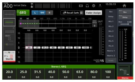
The current gain setting for each band is applied to the faders in the channel strip section on the top panel. You can confirm the frequency and gain applied to each fader in the channel name area of the display.
