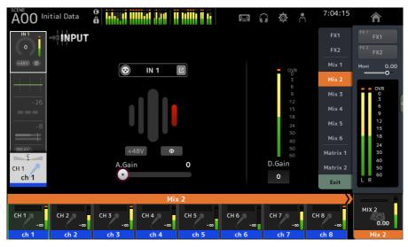
It displays channel names of the send to bus at the top of the channel name area.
