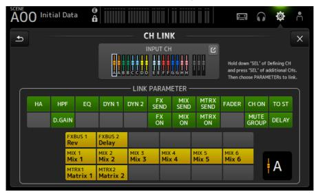
2 While pressing the [SEL] key of the link source of the input channel, press the [SEL] key of the link destination to link the channel.
