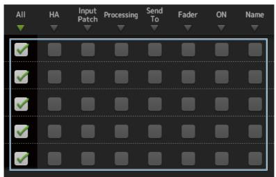
**3** To turn the recall safe ON for the selected channel, turn its SAFE button ON.
