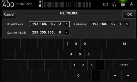
• Set different subnets for For Mixer Control and For Device Control.
