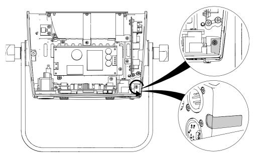
Unscrew the screw and remove the antenna cover.
