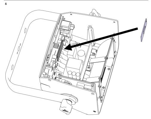
Finally, attach the TIMO board using the appropriate connector, and reassemble the cover by screwing all the screws back in.
