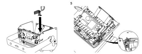
Secure the antenna in the space provided and screw in the 2 screws in Figure 5.
