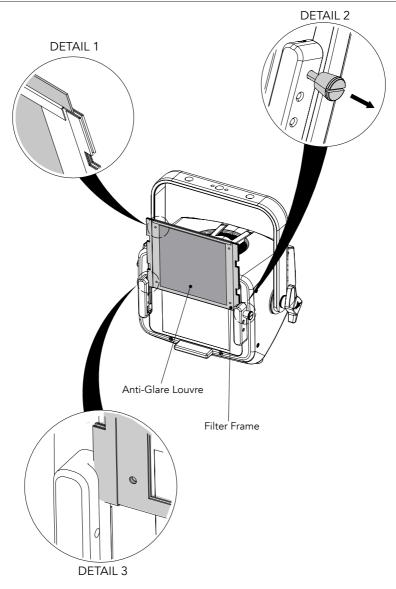
Insert the anti-glare louvre into the slot (DETAIL 1). Pull the knob out (DETAIL 2) and insert the accessory filter frame from the top into the guide on the hardware of the unit (DETAIL 3). Then release the knob (DETAIL 3).
