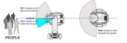
SHOW4 / Stage Hung : used when the fixture is fixed on stage, under the ceiling.
