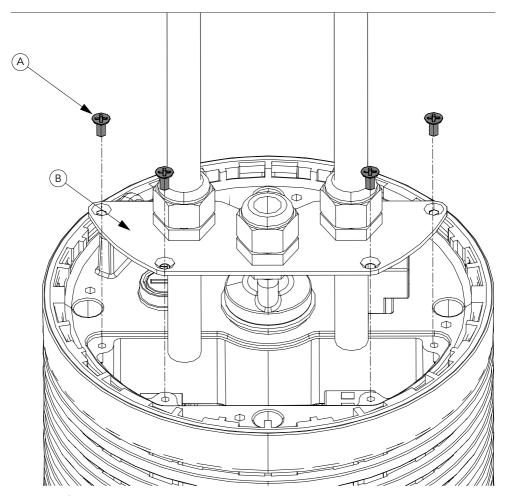
Loosen the four screws (A) and remove the plate with the cable glands (B). Then insert the cables.
