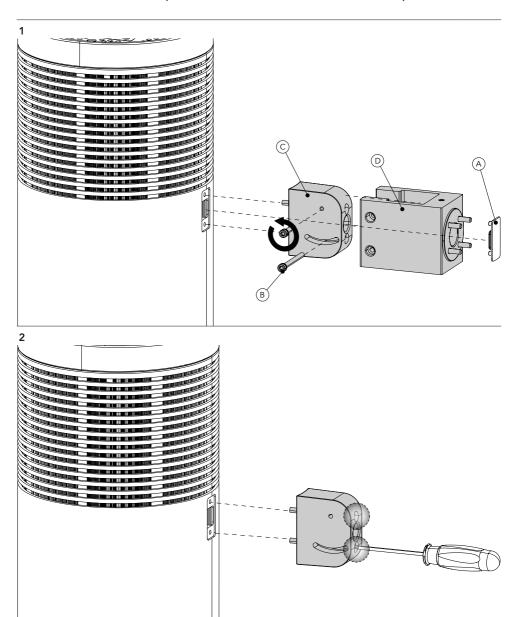
Remove the rubber from the desired side (A).
