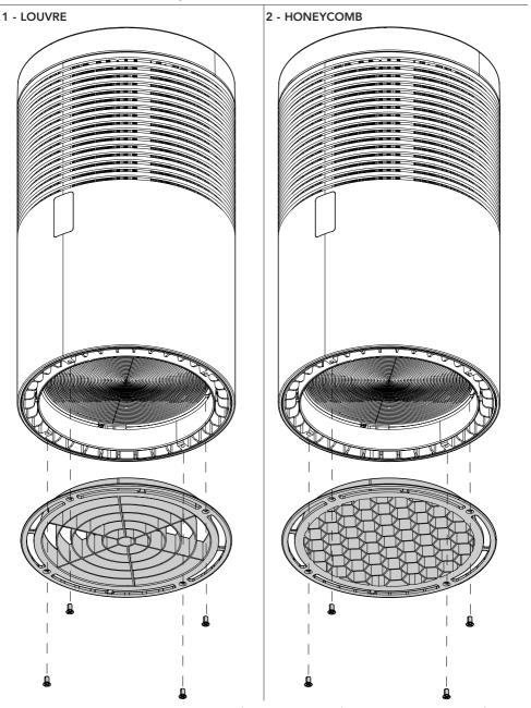
Attach louvre / honeycomb accessory to the fixture lens holder frame and secure with the four M4 screws.
