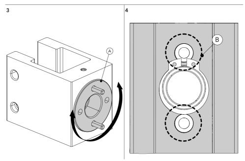
Rotate the disc (A) and align the two holes (B). Then insert the screws for wall fixing, and rotate it 90° again and insert the other two screws. Tighten the four screws in total.
