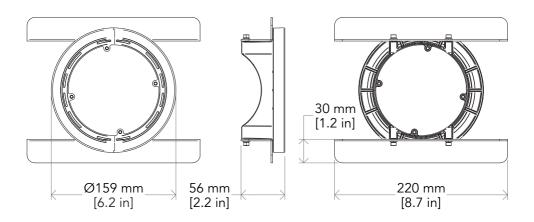
Measurements for cuts on the panels (A) and of Ceiling Mounted kit (B).
