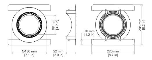
Measurements for cuts on the panels (A) and of Ceiling Recessed kit (B).
