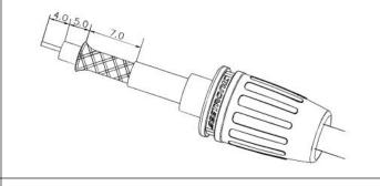
(3) Insert the pin into the center conductor of the coaxial cable. The tail of the pin should be fixed on the plane of the internal insulation layer of the coaxial cable. Use a crimping tool to compress the pin in the center conductor
