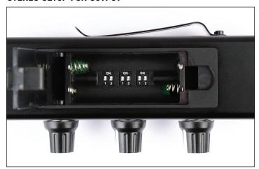
Using DIP switches inside the PX, each of the three channels can be independently sent to the left or right side of your in-ears/earphones/headphones, or both sides. This can help separate the different sound sources and make them easier to hear.
