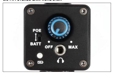
PX delivers impressive headroom, making sure you always have the volume you need—with your favorite in-ear monitors, earphones or headphones plugged into the top-mounted, standard 3.5 mm (1/8") stereo output jack.
