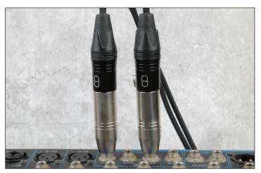
The XLR input plugs can accept balanced line signals taken directly from your mixer's aux outputs or main output. For 1/4" aux outputs, use the included XLR-balanced-to-1/4"-unbalanced adapters. This also works with headphone outputs, drum machines, audio interfaces, or any other audio device with a 1/4" output.
