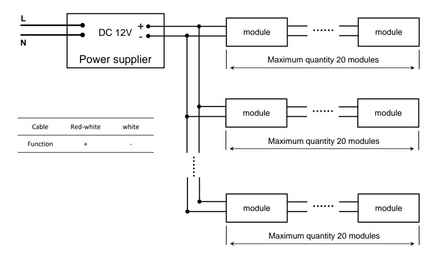
\* The secondary cable recommend > AWG18, < 3 meter
