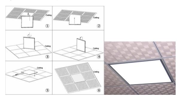
1, Make sure the panel light work well before installation then put the panel light at the diagonal position.
