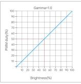
Linear dimming curve
