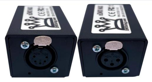
5pin and 3pin XLR socket variants. DMX port status indicator bottom left of XLR socket.
