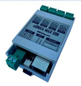
Network 10/100Mbps RJ45 socket. Pluggable 2way 5mm pitch terminal block for 7-28Vdc power input. Four 3way 3.5mm pitch pluggable terminal block connectors for DMX512.
