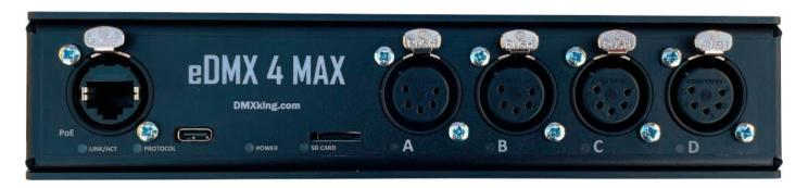
Power over Ethernet 802.3af / network 10/100Mbps RJ45 Ethercon socket. USB-C socket for DC power input alternative to PoE. SD card push-push socket for microSD. Four Neutrik XLR connectors for DMX512 3pin or 5pin options available.
