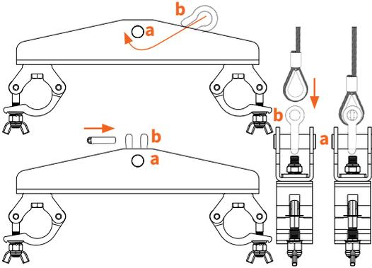
Alternatively, connect the TRUSS BRACKET 30/40HC to the lifting hook. Open the hook, place the pin (a) of the TRUSS BRACKET 30/40HC in it and secure the hook again.
