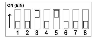
Therefore, to create an opening time of 400ms the switches 3 and 5 must be set to "ON" and all others to "OFF".
