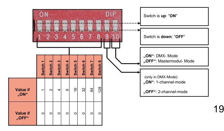
The dip swith has 10 single switches (see picture above). The switches 1-8 (from left) allow you to set the opening time in mastermodule mode, or the DMX channel in DMX mode. Switch 9 is used to change between 1 channel DMX mode (only ignition channel) to 2 channel DMX mode (ignition and safety channel). Switch 10 allows you to select between DMX or mastermodule mode.
