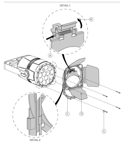
Push the screw (A) and and open upward the gel frame lock (B) provided on the holder (C). Insert the barn doors (D) from above by inserting the linking holders into the guides (DETAIL-2) of the holder (C).Mount the assembly at the four holes provided on the unit with the screws. Then close the frame lock gel.
