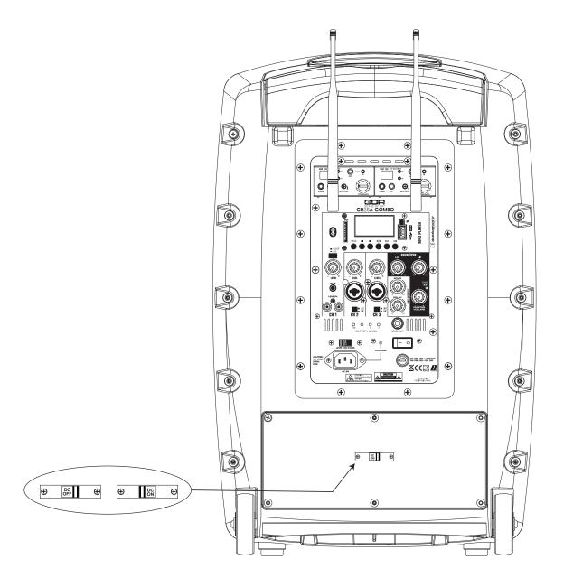
The switch on the battery door allows the batteries to be disconnected. Turn it to the DC ON position before charging your device for the first time. Turn it to DC OFF if you do not use your device for a long time.
