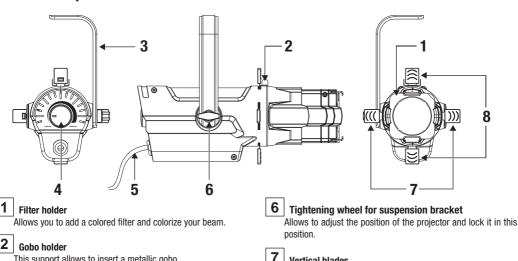
This support allows to insert a metallic gobo.
