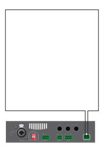
The installation consists of an electrical wire that runs through the perimeter of the room forming a loop.
