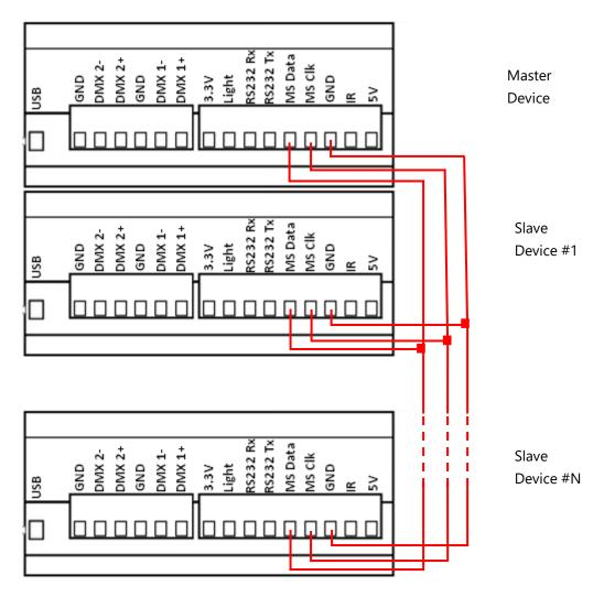
Interfaces configured as slave will strictly follow the clock, triggers and information providing by the master interface. Only one master interface at a time is possible.
