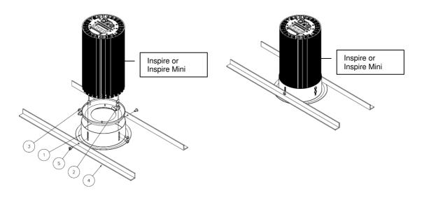
Caution: The angle supports of the ceiling installation kit must be mounted or attached to the ceiling with the appropriate load capacity.
