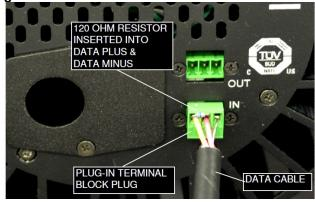
**Figure 6 Data Cable Termination**
