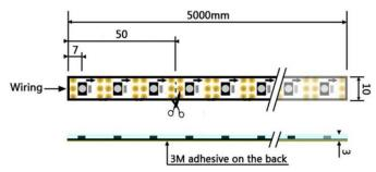
• 50mm spacing between each cutting point.
