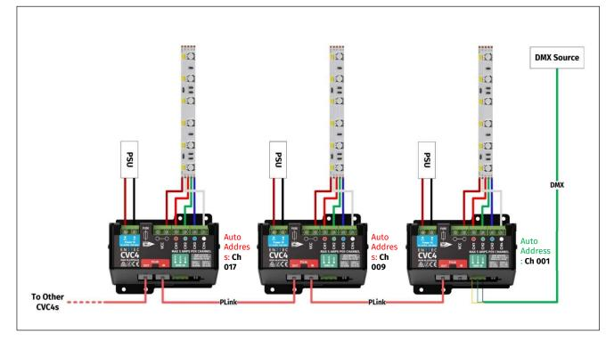
Note: The CVC4 allows for operation mode to be set by DIP Switches only - Not via RDM.
