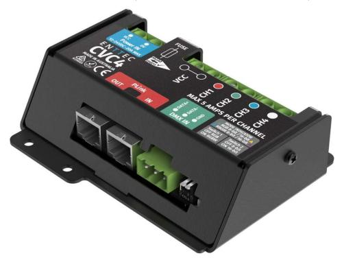
ENTTEC's CVC4 is a high precision 4 channel, constant voltage (CV) LED dimmer, capable of dimming up to 5A of LED tape per channel at 12-24v.
