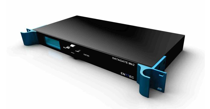
The Datagate is an extremely powerful and flexible bridge between controls and any DMX512 device. It can form the backbone of a network, provide optical isolation, merge levels from multiple streams, translate between DMX and Ethernet protocols and even play back Architectural lighting shows.
