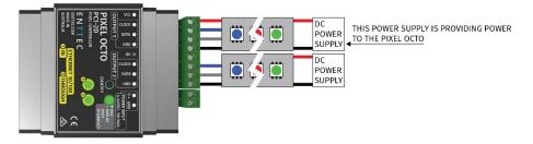
POWER CONNECTION (USING TERMINAL SPLITTERS)
