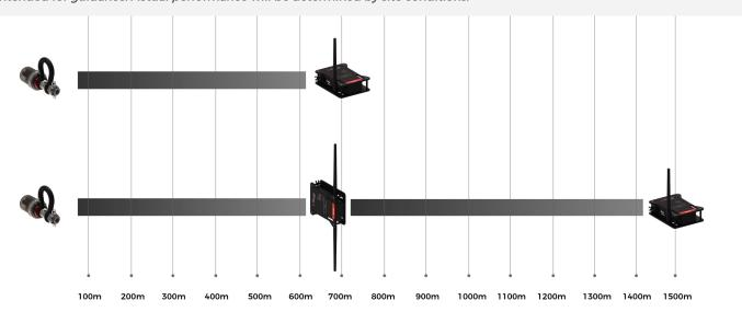
In case it is necessary to cover longer distances or there are large obstacles to overcome, it is possible to add Repeaters, which can be located as far as 600 meters from the cells and 700 meters from the Cateway. It is not possible to connect multiple Repeaters in series: each Repeater needs a direct connection to the Cateway.
