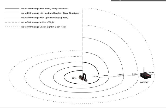
The maximum range of any wireless system depends on the propagation conditions: If the propagation between the cell and the Cateway is in line of sight, the maximum range achievable with our system is about 600 meters. In the graph we have simulated the limitations due to various types of obstacles. Data are taken from field tests and theoretical calculations and are intended for guidance. Actual performance will be determined by site conditions.
