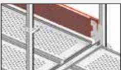
Assembly of the wooden toe board
