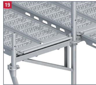
19 0.7m bracket cantilever using Allround bracket, bracket brace and scaffolding decks.
