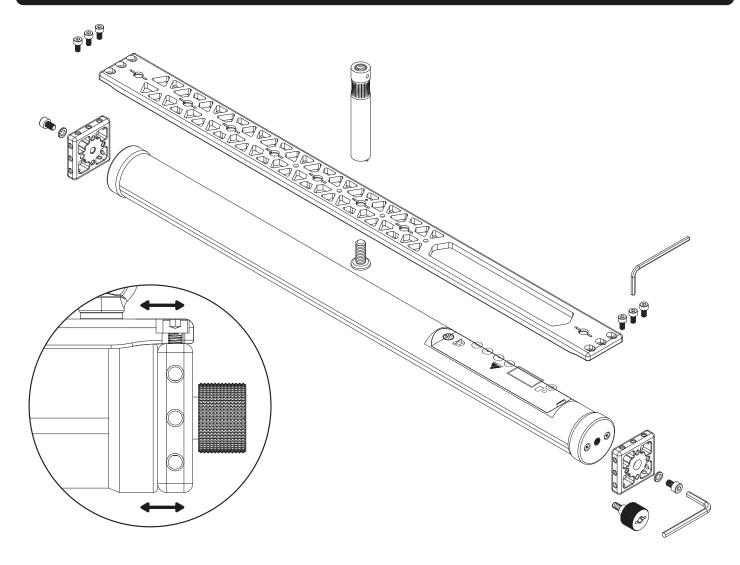
To mount the Exo Bone Kit on the Astera tube, mount the two Exo Slabs on both sides with the 3 +3 Allen screws (do not tighten the screws), then install the Exo Pin and then the Astera tube.
