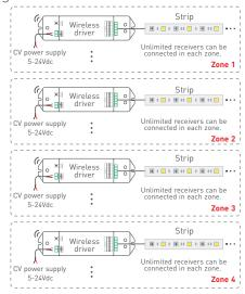
To avoid the signal interference, the installation needs to keep away from the large area metal material or the metal material space.
