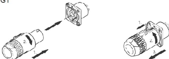
Insert the male speakon in its corresponding hole and turn right until it clicks. This fixes it safely and strongly and helps stop it being pulled out by mistake. At the other end of the cable connect in the same way to the amplifier channel.
