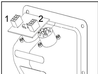
Change the cable from one plug to the other and screw the connector panel again. That's all.
