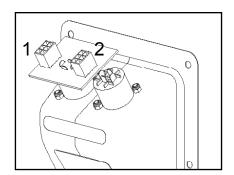
Change the cable from one plug to the other and screw the connector pannel again. That's all.
