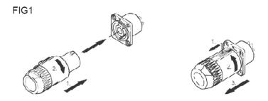
Insert the male speakon in its corresponding hole and turn right until it clicks. This fixes it safely and strongly and helps stop it being pulled out by mistake. At the other end of the cable connect in the same way to the amplifier channel.
