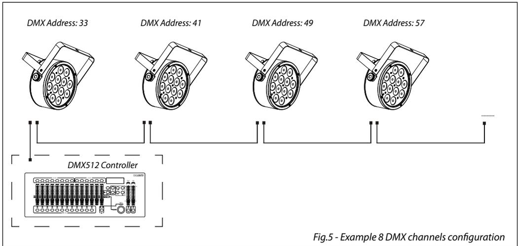
Fig.5 - Example 8 DMX channels configuration
