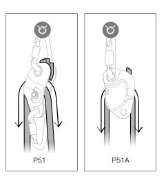
• With the cam activated, make sure the rope circulates in one direction and locks in the other direction.
