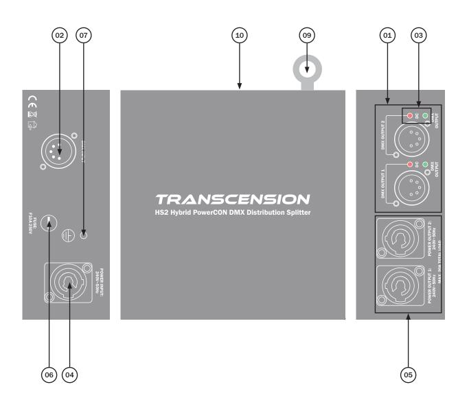
01 - 2 x 5-Pin DMX outputs 02 - 5-Pin DMX input 03 - DC/DMX output indicators
